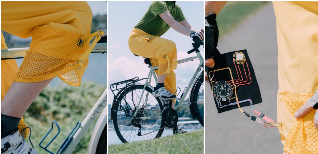
Fig 1. High Water Pants mechanically shortened showing a cyclist is in an area in Seattle that will be impacted by sea level rise in the future (left) in the ‘down’ position (center) and showing the microcontroller soft circuit (right).
