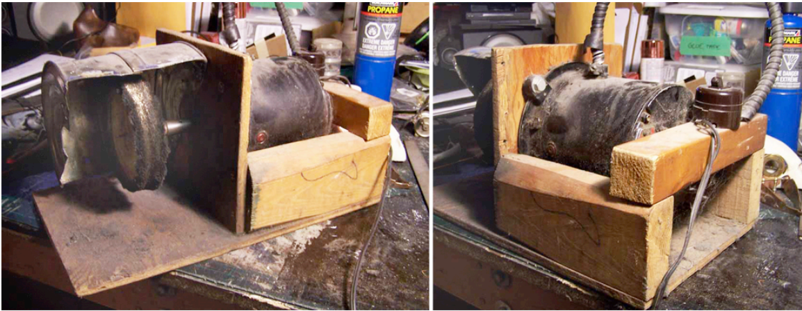
Figure 19. Homemade polishing machine (images by Adrian)
