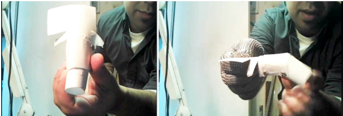
Figure 24. Kenneth's Bristol cardboard prototype, planning for cutting copper sheets. (images by Audrey Desjardins)
