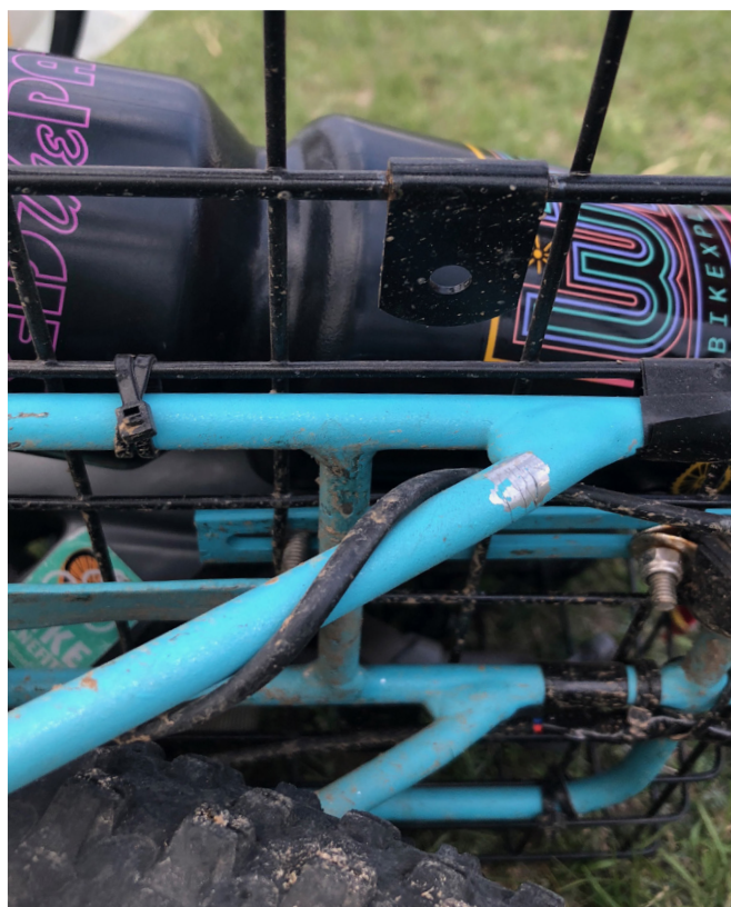
Figure 7. Site of repair: A cracked and bent front rack caused rubbing on the tire, Rep(AIR) diffused cinnamon to communicate the impact.
