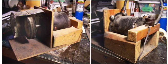
Figure 5: Homemade polishing machine.
