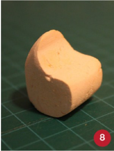
Figure 5. A yam potato used as prototyping material.
