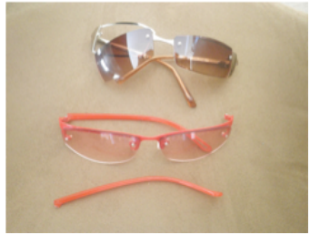
Figure 2. Substitutable Materials: These broken sunglasses (with missing screws) were repaired by taking screws from an extra pair and substituting them in the broken pair.
