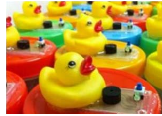
Figure 1. Flood Ducks detect voltage in flooded homes.
